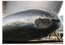
Figure 4: Lead keel impact - That should buff out!
